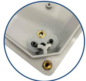
Tip: Panel mount is secured when set screw tip is flush or extends past the bottom of the pad about 1/16"
