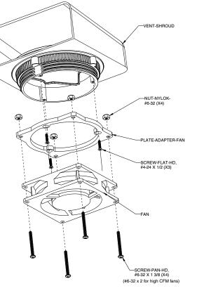
TIP: When installing a forced air solution, a second Fan Shroud or Vent should be installed to allow free air movement.
