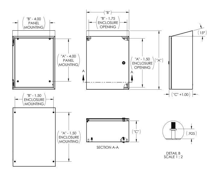
Submit drawings to customerservice@integraenclosures.com for approval and quote. \*Unless otherwise specified, our standard gauge size for enclosures 20"x20" and smaller are 16 gauge. For enclosures 20"x20" and larger, our standard is 14 gauge.
