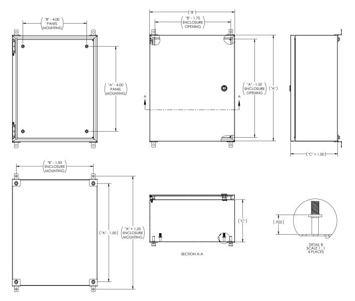
Submit drawings to customerservice@integraenclosures.com for approval and quote. \*Unless otherwise specified, our standard gauge size for enclosures 20"x20" and smaller are 16 gauge. For enclosures 20"x20" and larger, our standard is 14 gauge.
